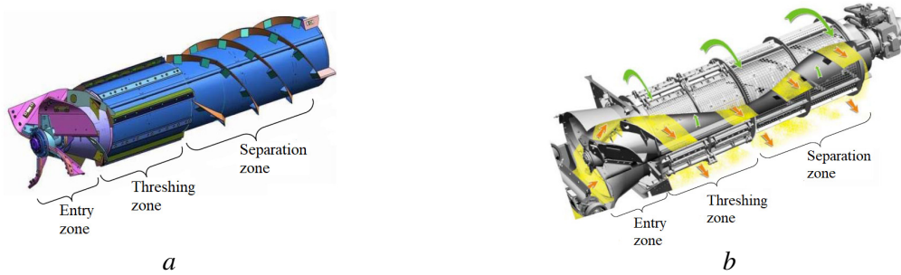
Fig. 4. Rotary threshing-separating device of combine harvester Rostselmash Torum: a – rotor; b – rotor-deck system
