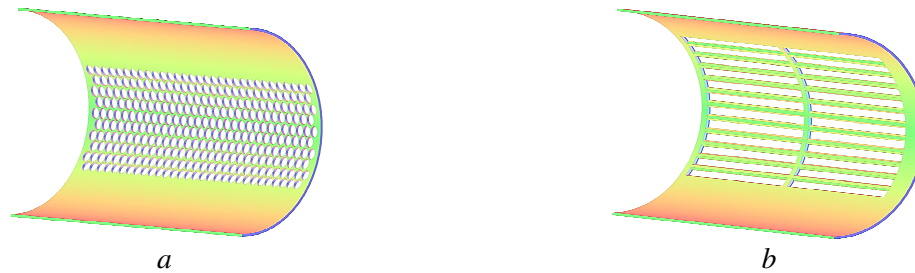
Fig. 6. Part of deck of experimental rotary threshing-separating device: a – smooth sieve; b – relief sieve
