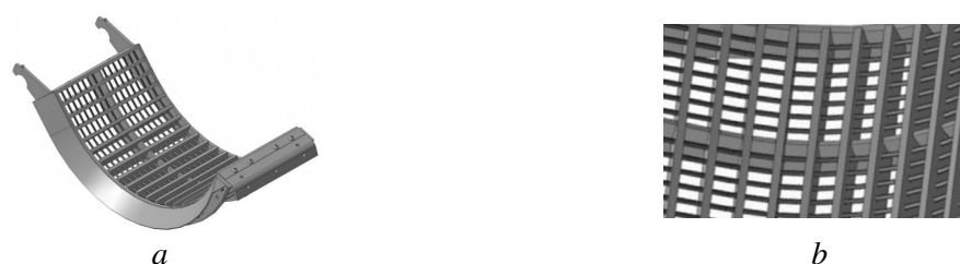
Fig. 3. Design sections of deck rotary combine harvester: a – deck section; b – relief of the internal surface of the deck
