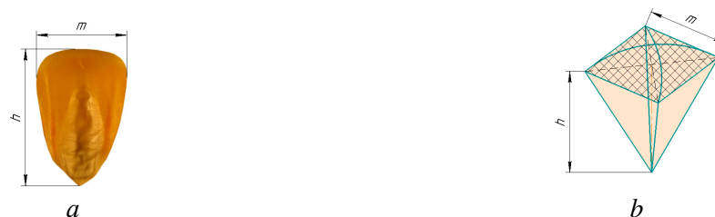
Fig. 2. Parameters for determining calculated grain diameter: a – corn grain; b – grain model
